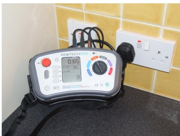
Using a multifunction meter to check Earth Fault Loop Impedance
