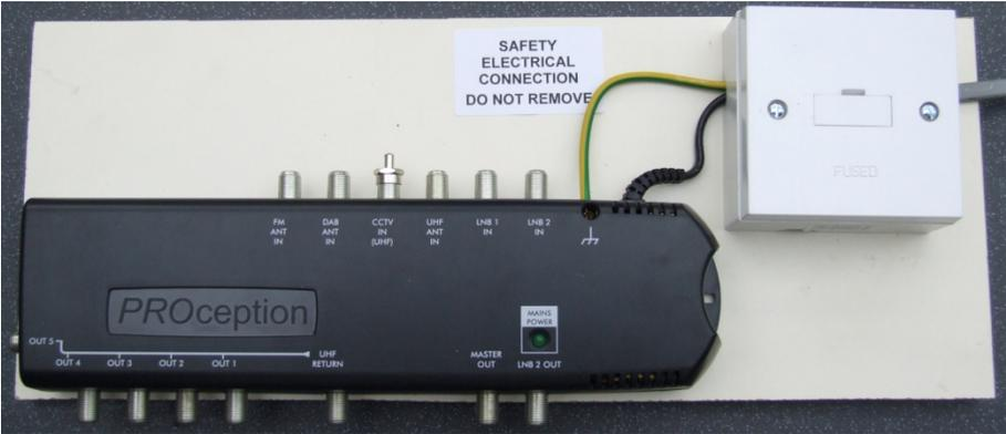
Connecting to the earth tag on an amplifier from a fused connector unit
