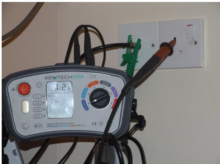
Doing a final resistance test between the outlet and a convenient local earth.
